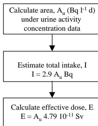
Figure 0-2. Direct dose method for intakes of tritiated water
