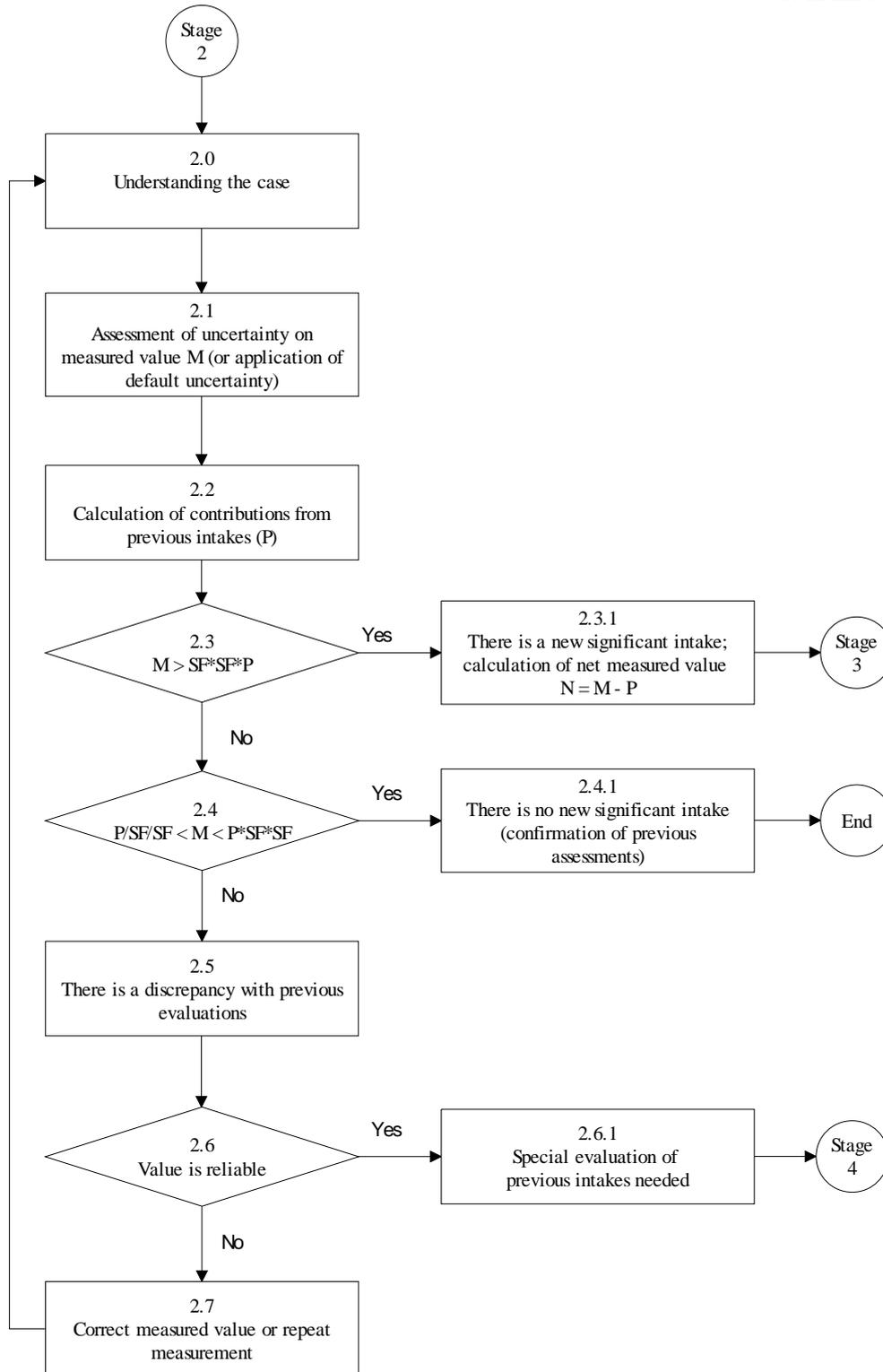
Fig. 8.2 Stage 2 – Structured approach to dose assessment. Check on significance of new measurement and consistency with previous evaluations. (M – measured value, SF – scattering factor, P- contributions from previous intakes – see text)
