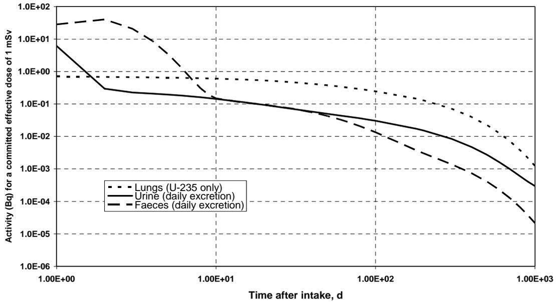
Fig. A27.3. Inhalation Type S: predicted activity of U-235 in lungs and U-234 or U-238 in urine and faeces following acute intake of natural U
