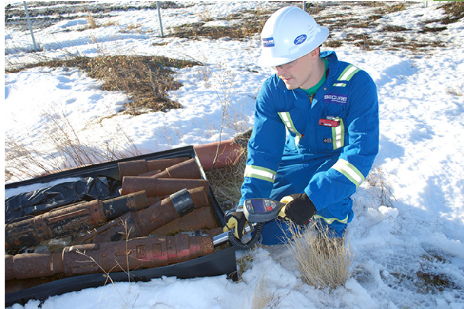
A SECURE NORM technician is conducting a NORM screening survey on down-hole tubing and equipment prior to release from location.
